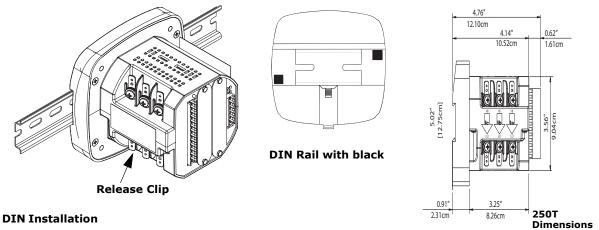
**Installation Steps:** Slide top groove of meter onto DIN Rail. Press gently until the meter clicks into place. If mounting with DIN Rail provided, use Black Rubber Stoppers (also provided) shown above. To remove meter, pull down on Release clip.
