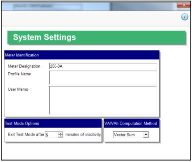
2. Input a new meter designation into the field. Note that it is important to name each meter individually, since the meter name is used to name the log databases when logs are downloaded. See Chapter 28 in the software manual for an explanation of the other settings in this screen.
