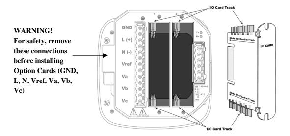
3. Slide the card inside the plastic track and insert it into the slot. You will hear a click when the card is fully inserted. **Be careful**, it is easy to miss the guide track.
